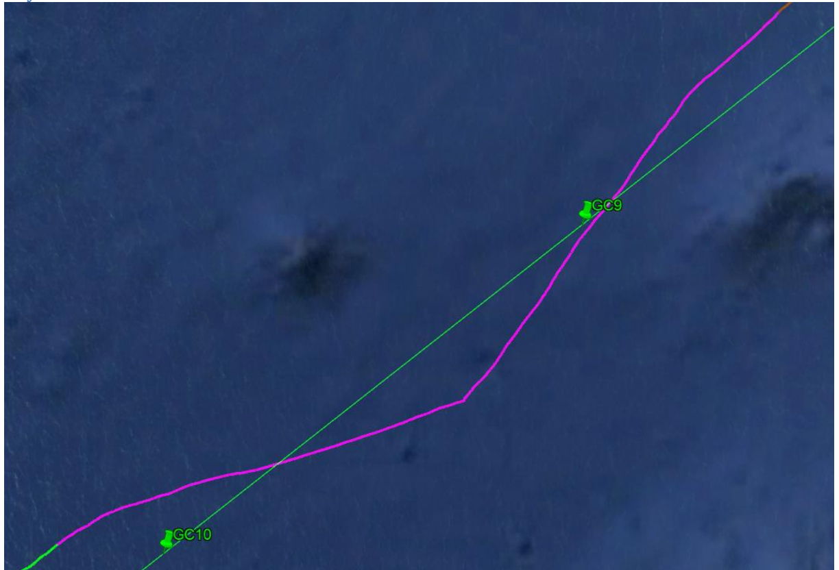
Image 51 Route planned (green) and real track (purple) of day 6. Etmal was 126nm, distance between GC9 and GC10 is 70nm, max XTE 9,5nm.
