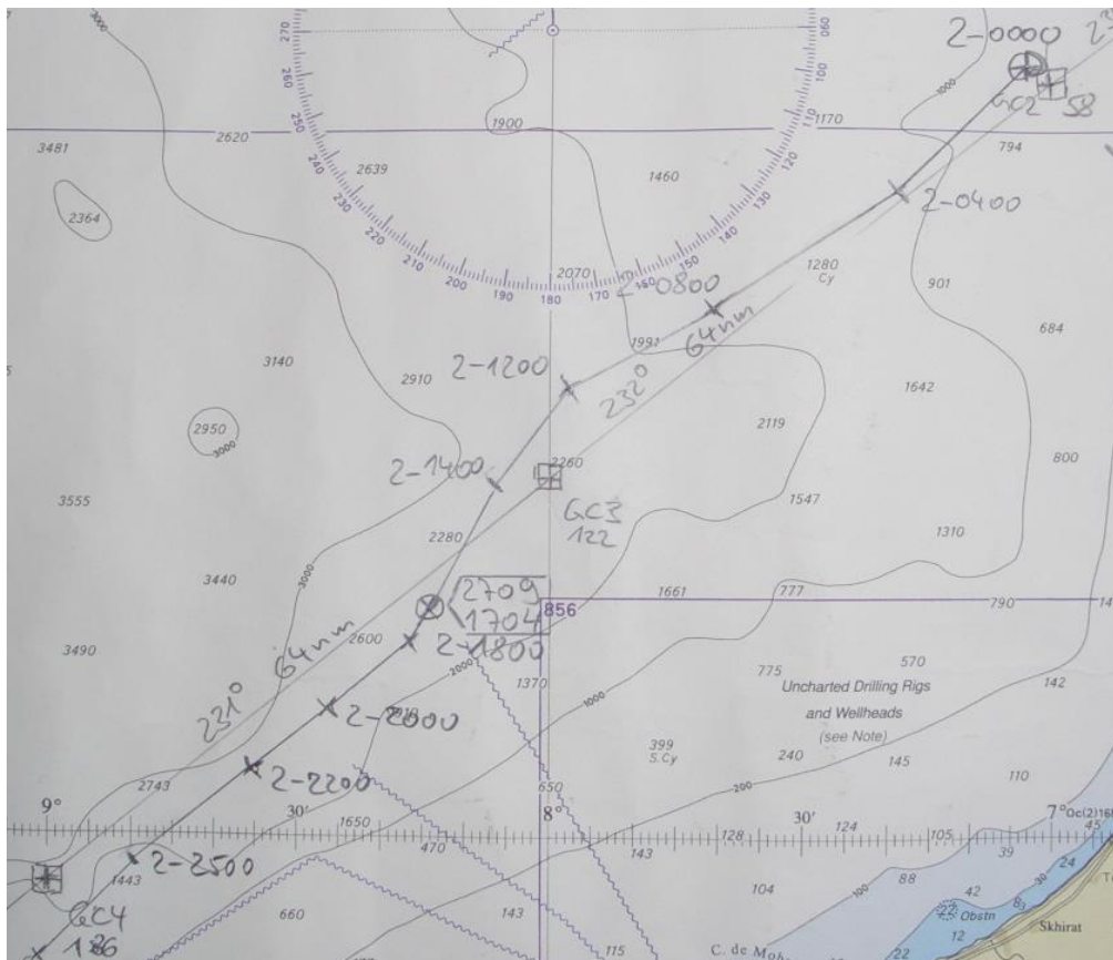
Image 36 Dead reckoning of day 2 started at fix 2-0000 with a fix at 1704BT (1604 UTC)
