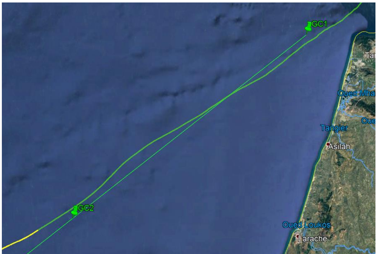
Image 31 Route planned (green thin) and real track (green thick) of day 1. Etmal was 103nm (in 17,5 hours!), distance between GC1 and GC2 is 55nm, max XTE 2,4nm.
