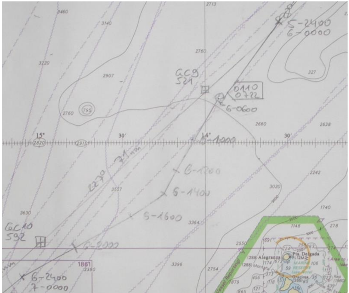
Image 52 Dead reckoning of day 6 started at DR 5-2400 with a small correction fix at 0722BT (0622 UTC)
