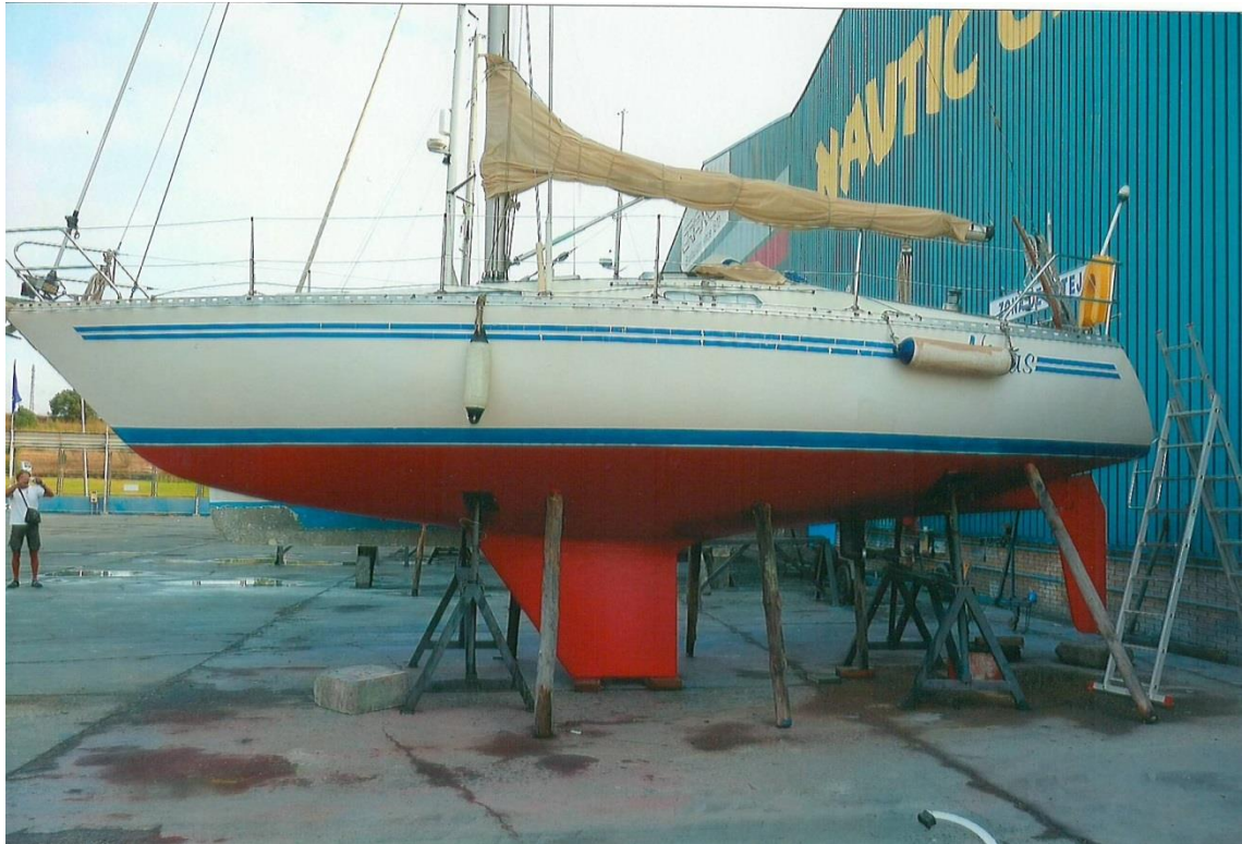
Image 7 Nicas lateral plan, a fin keel with sail drive and a spade rudder protected by a small skeg.
